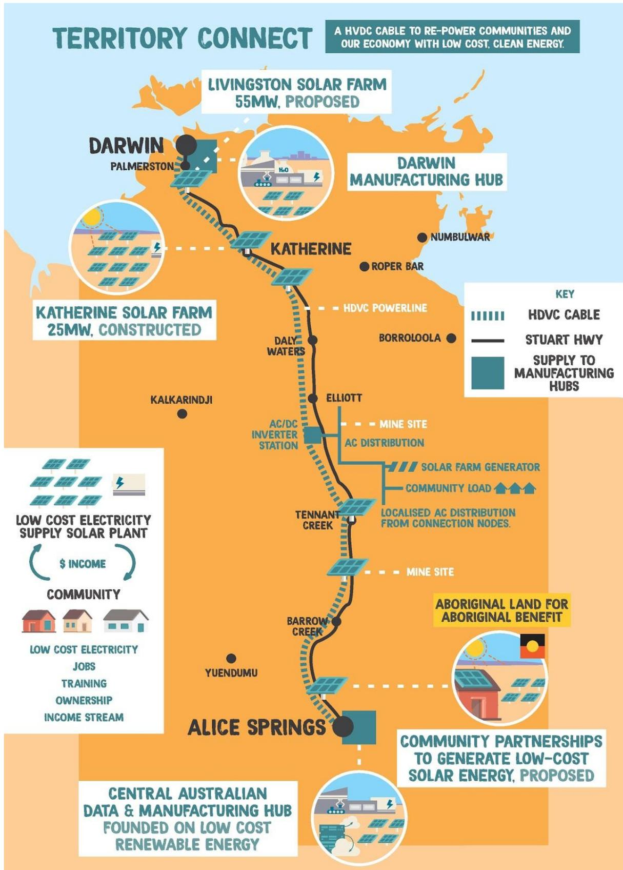
**Image:** The proposed 'Territory Connect' HVDC transmission link connecting Darwin to Alice Springs.
